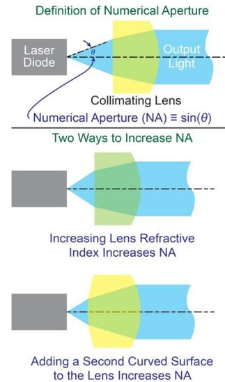
**Fig 1. For a lens of a given shape, a higher index material will produce a shorter focal length and higher NA. Alternately, without changing material index, using steeper curve(s) on the lens surface(s) will reduce focal length and increase NA.**
