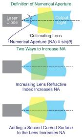
Fig 1. For a lens of a given shape, a higher index material will produce a shorter focal length and higher NA. Alternately, without changing material index, using steeper curve(s) on the lens surface(s) will reduce focal length and increase NA.
